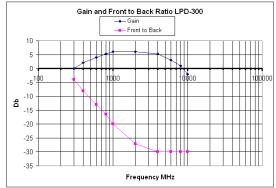
The LPD-600 and LPD-300 are lightweight, medium-gain, log periodic antennas manufactured on FR4 .063" fiberglass board. They have a useful frequency range of 300 MHz to 18 GHz and receive linear polarized radio waves. The antennas have an SMA connector and incorporate a handle, cable strain relief, and ½"-20 threaded insert for mounting on a camera tripod.
